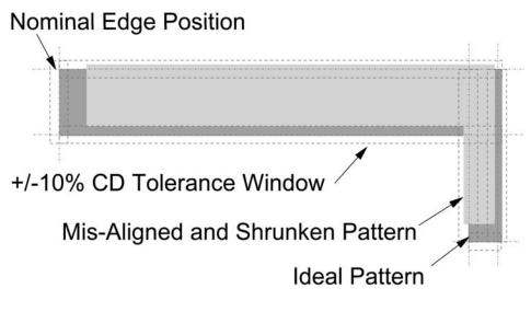
Figure 1.4 Edge placement tolerance.
