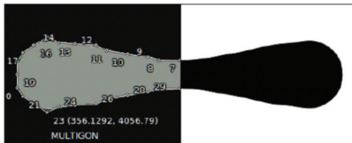
Figure 9. Symmetrical MULTIGON record displayed by design data viewer (left) and rasterized image by ACTIS with the developed SEMI P49 OASIS-compliant engine (right).
