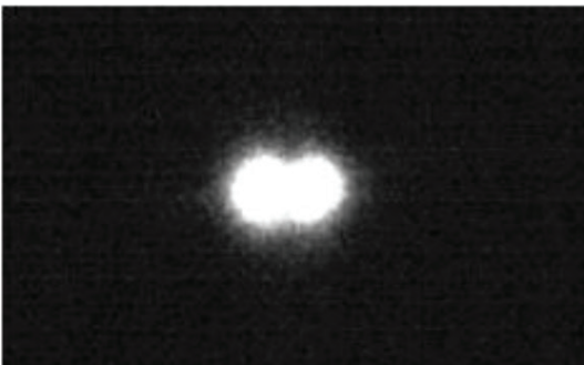
Figure 14. Plasma shape of the EUV emission area. Size is 90 micrometers by 45 micrometers.
