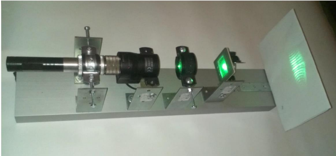
Ronchi interferometer made by Oleksandr Malenko
