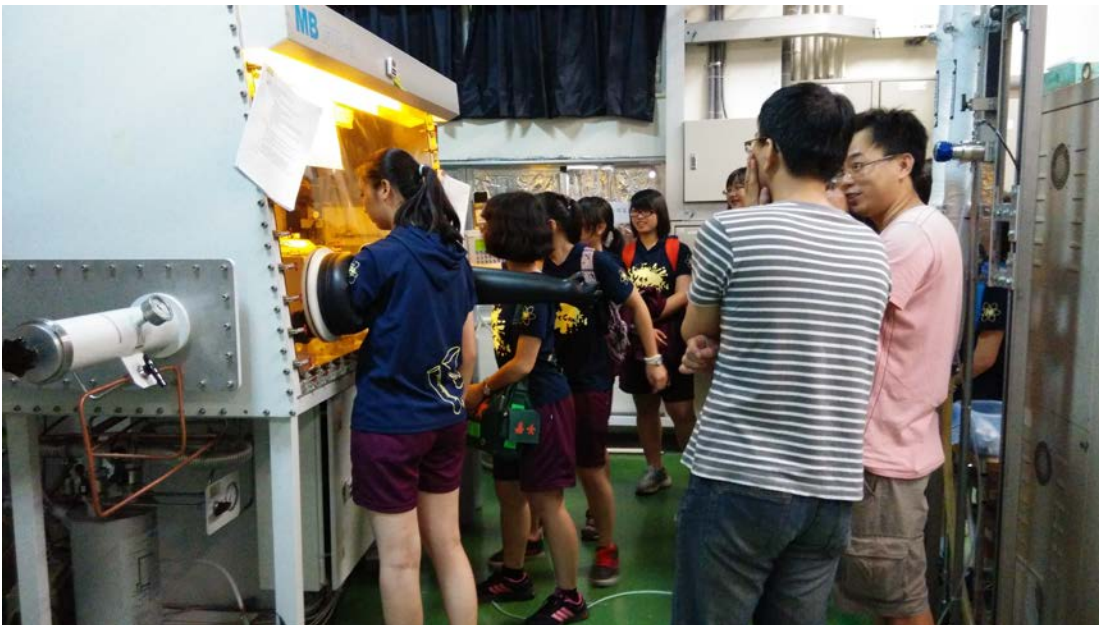
Fig.7 photo of CYGH's students visiting the public laboratory and learning to use the nitrogen gas holder. That was used to manufacture OLED and some devices that need low-oxygen environment.
