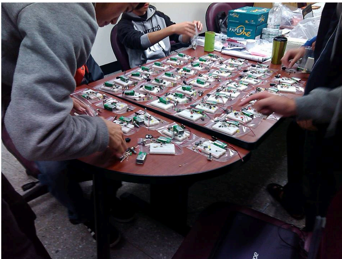
Fig.1 photos of the staff preparing the materials of simple hand-made electrical candle, that the LEDs on it can cross flashing by using the charging and discharging effect of the circuit contains capacitances, resistances and LEDs.
