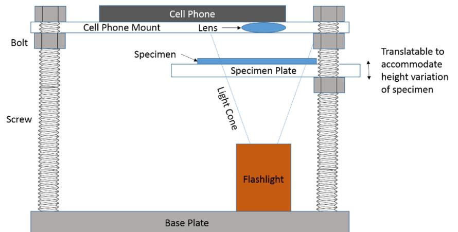
built more as an add-on to cell-phones, which is ubiquitous among students today, and allowed imaging of micro-structures with minimal additional cost/components. We show a brief schematic of this microscope to the right.
