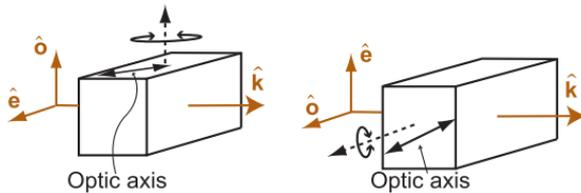
Another important consideration when working with a mixture of e- and o-waves is **Poynting vector walk-off**  $\rho$ . In many cases, walk-off limits the effective crystal length since the interacting beams physically separate.
