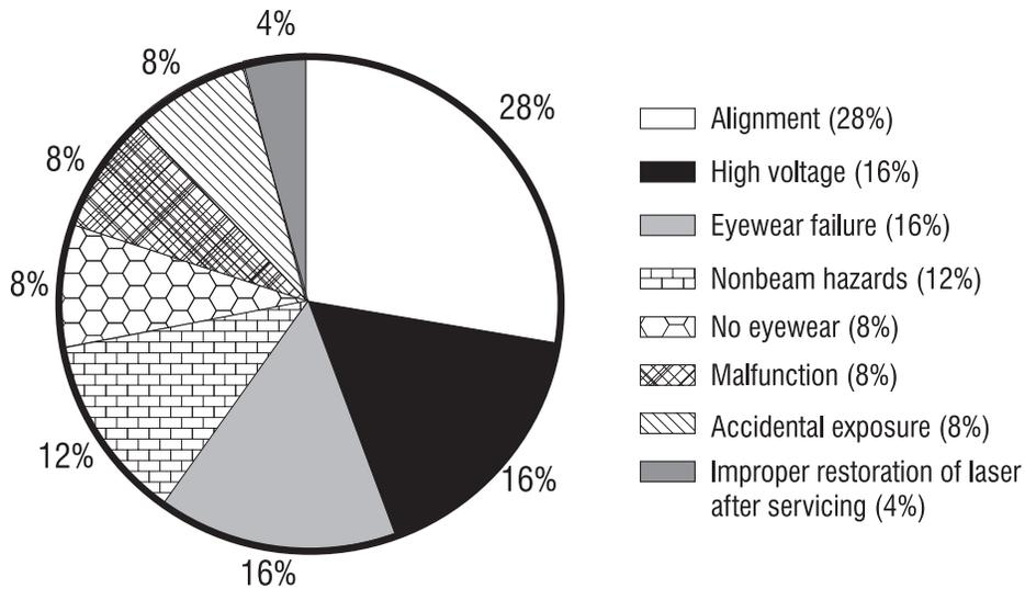
**Figure 2-18** *Causes of most laser accidents*
