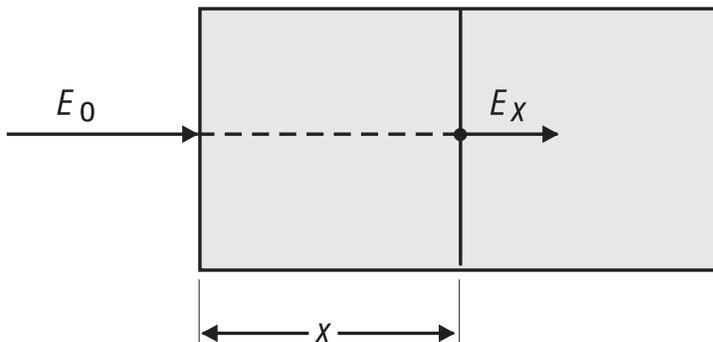
Figure 2-15 Absorption of light in transparent materials
