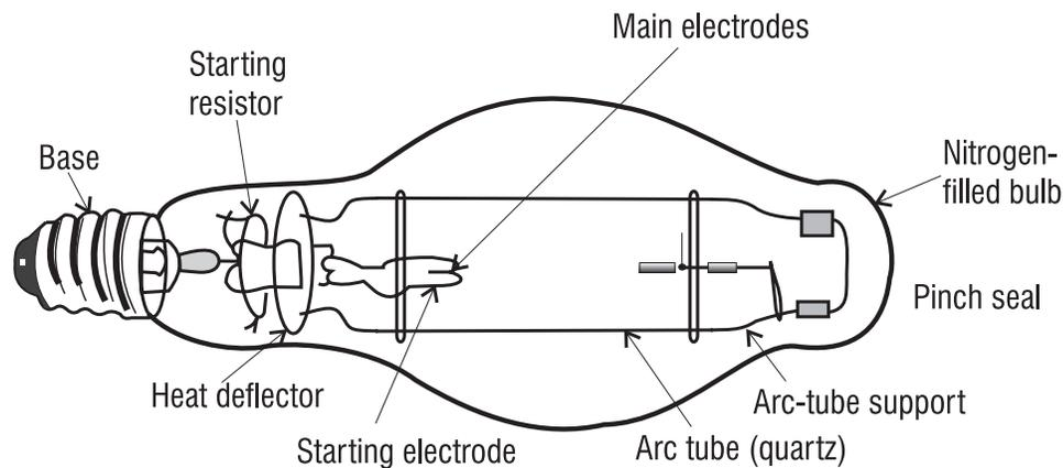
**Figure 2-6** Mercury HID lamp. This cutaway drawing shows the construction of an Hg-HID lamp. The inner envelope is of quartz; the outer envelope of borosilicate glass (adapted from Kaufman and Christensen, 1972).
