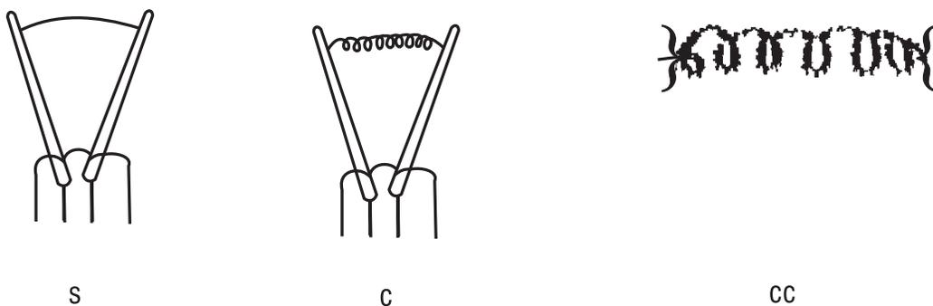
**Figure 2-5** *Types of incandescent filaments. Filaments are arranged upon support structures within the bulb in a variety of ways. The filament itself may be either straight (s), coiled (c), or coiled coil (cc).*
