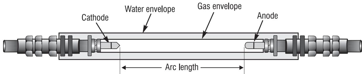
**Figure 2-7** Diagram of a gas arc lamp with water jacket for cooling
