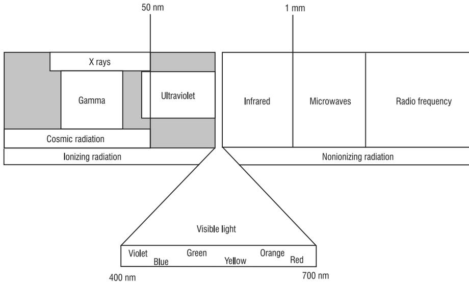
**Figure 2-11** Important regions of the electromagnetic spectrum
