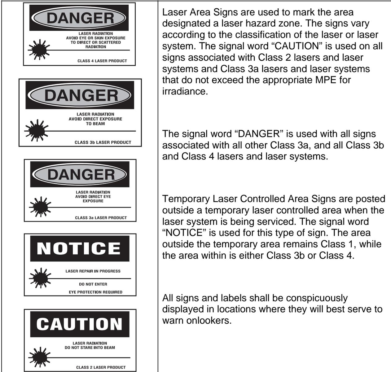
Laser Area Signs are used to mark the area designated a laser hazard zone. The signs vary according to the classification of the laser or laser system. The signal word “CAUTION” is used on all signs associated with Class 2 lasers and laser systems and Class 3a lasers and laser systems that do not exceed the appropriate MPE for irradiance.
