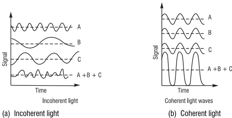
**Figure 2-4** Adding coherent and incoherent light waves
